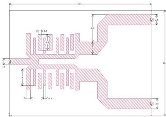
Figure 1: Top view of the Power Divider
