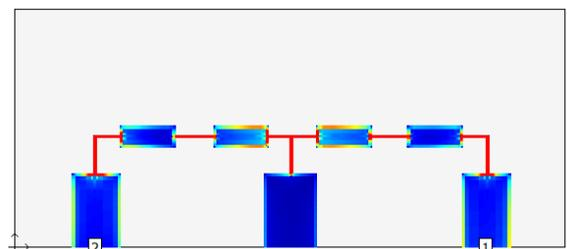
Figure 4: Current distribution at 7 GHz
