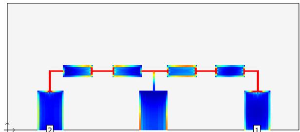
Figure 5: Current distribution at 11 GHz
