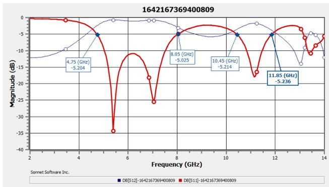
Figure 3: Filter response graph (S11 RED, S12 BLUE)
