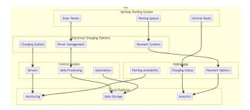
Block diagram of the Smart vertical parking system Challenges
