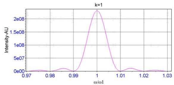
Figure 3(a) : Intensity of radiation at 1<sup>st</sup> harmonic
