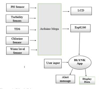
Figure 1. Block Diagram
