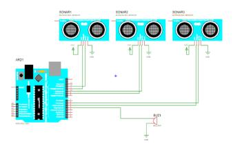
Figure 4. Wiring Diagram of Overflow Control
