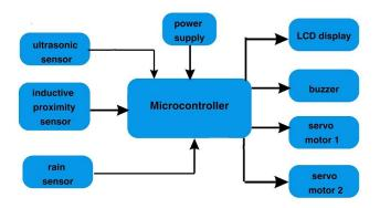
Figure 1. Block Diagram of Smart Waste Segregator
