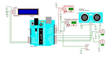
Figure 3. Wiring Diagram of Waste Segregator
